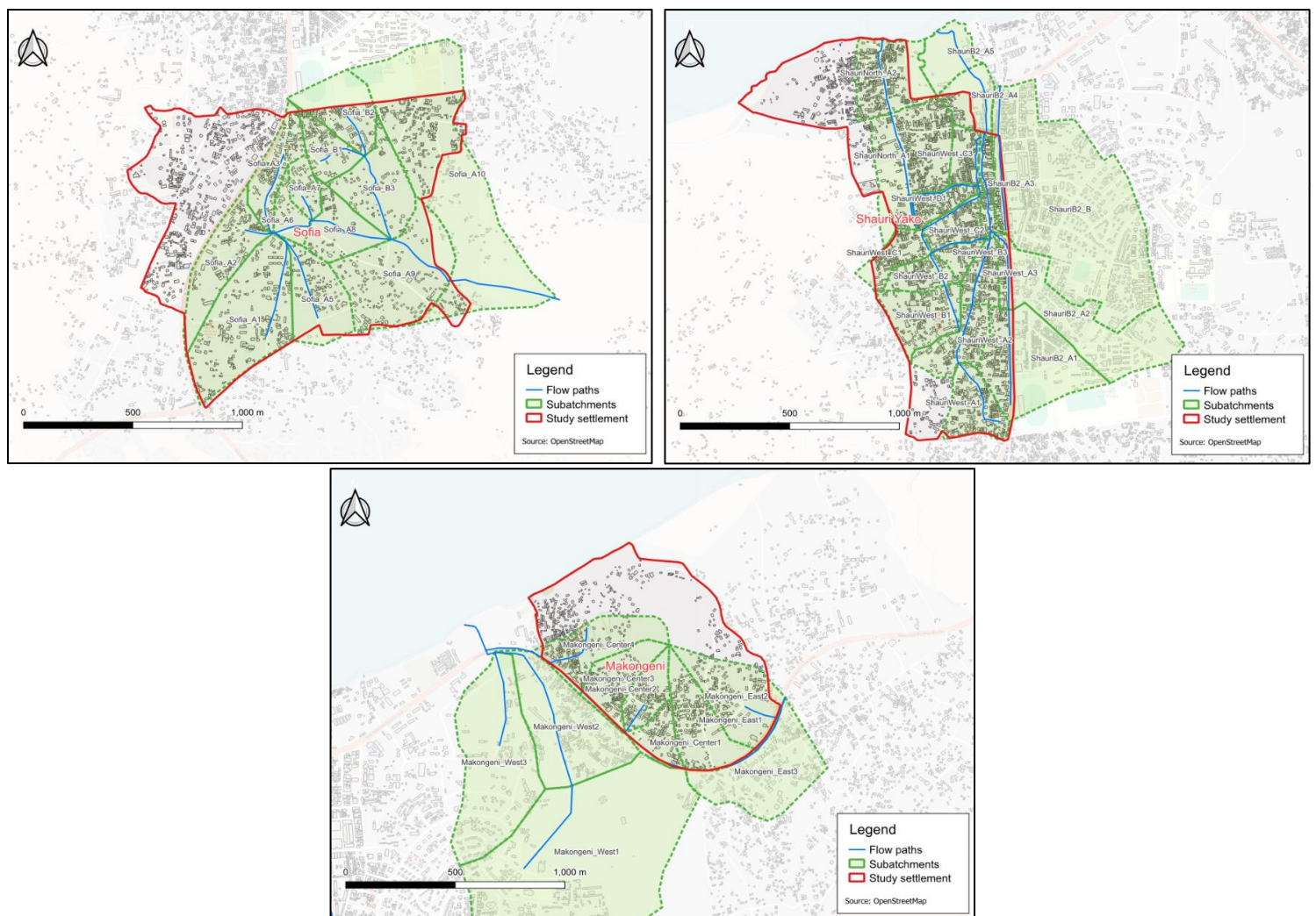
Figure 40: Sub catchments and flow paths for the three settlements (Source: SUEZ Consulting, 2025)
